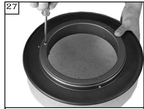
27 Remove 3 screws from the frame with the glass. Save these screws.
